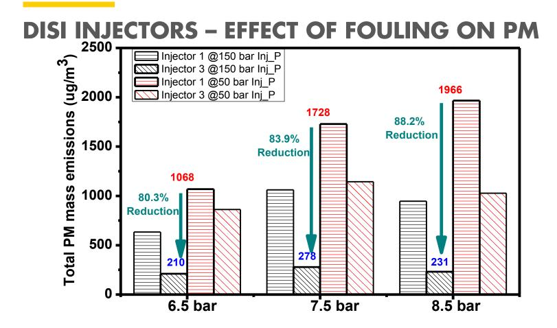
Injector 1= fouled injector with 8.5% flow rate loss Injector 3- new injector
