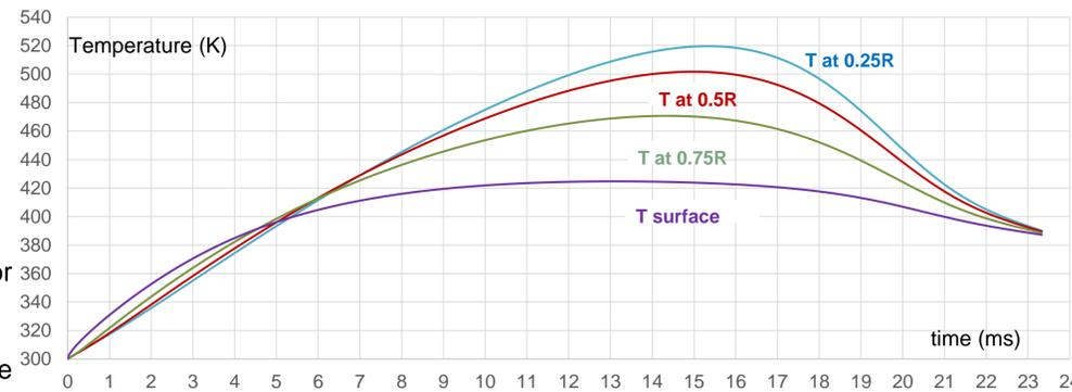
Heating and evaporation of n-heptane semi-transparent droplet under ETC model in the presence of thermal radiation from a flame. Thermal radiation temperature is 2200 K.
