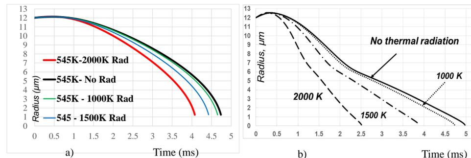
a) Radius ( $\mu\text{m}$ ) as function of time (ms) by SHRL\_ST code for n-heptane semi-transparent droplet
