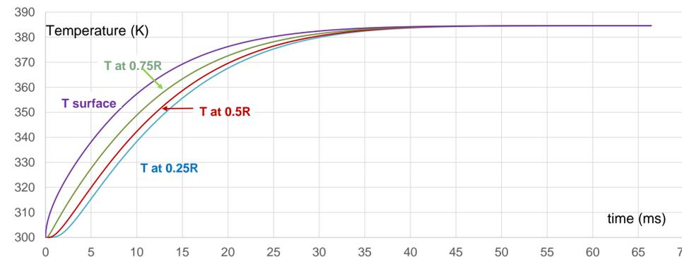
Heating and evaporation of n-heptane droplet under ETC model in the absence of thermal radiation
