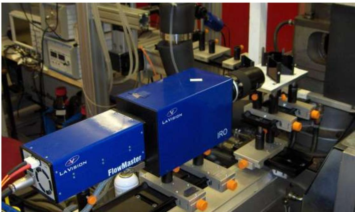
Figure 80 – Set of reflective filters in front of UV lens, intensifier and camera
