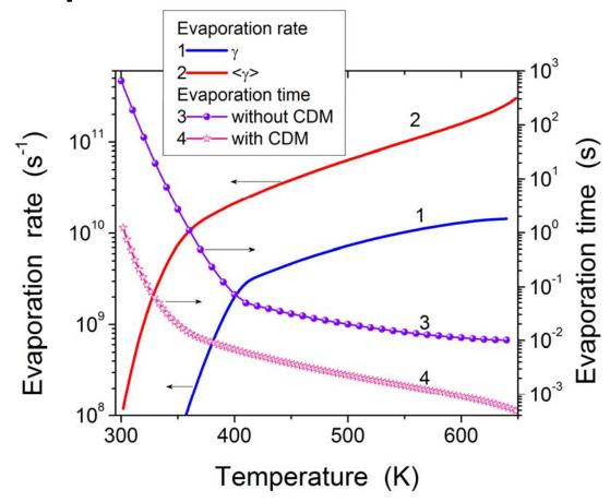
Comparison of the evaporation rate  $\gamma$  (curves 1 and 2) and evaporation time (curves 3 and 4 without condensation) of n-dodecane nanodroplet (droplet radius 2.65  $\mu$ m and number of molecules 1.46×10<sup>8</sup>, pressure 3.5 MPa) without (curves 1 and 3) and with (curves 2 and 4) taking into account CDM for 67 conformers calculated using  $\omega$ B97X-D/cc-pVTZ and SMD/ $\omega$ B97X-D/cc-pVTZ.
