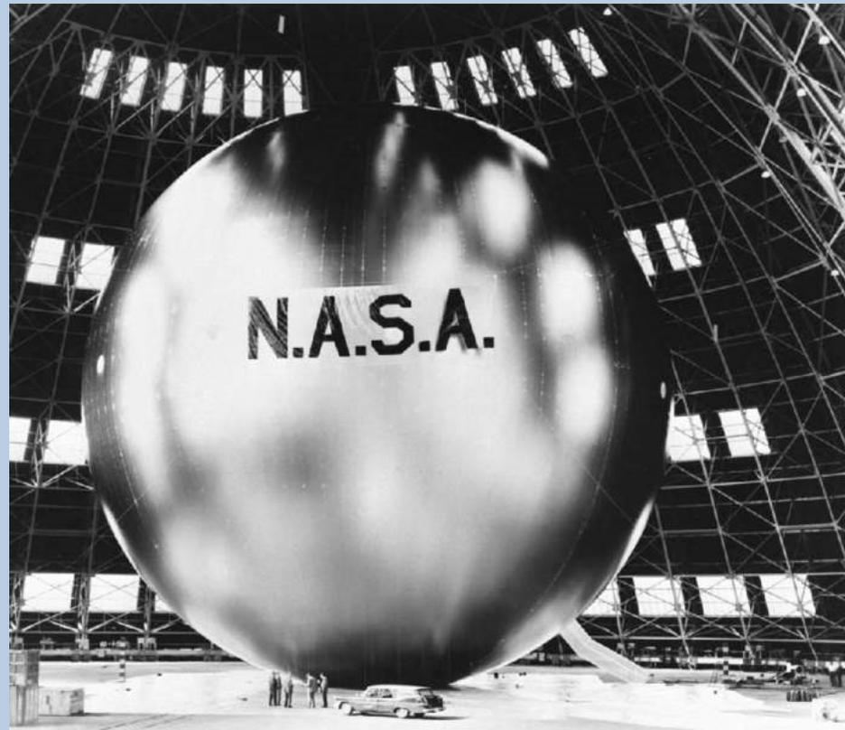
1960's: **NASA "Echo"** project for transmitting radio waves by satellites looking like a large sphere with thin wall from polymer material and aluminium skin
