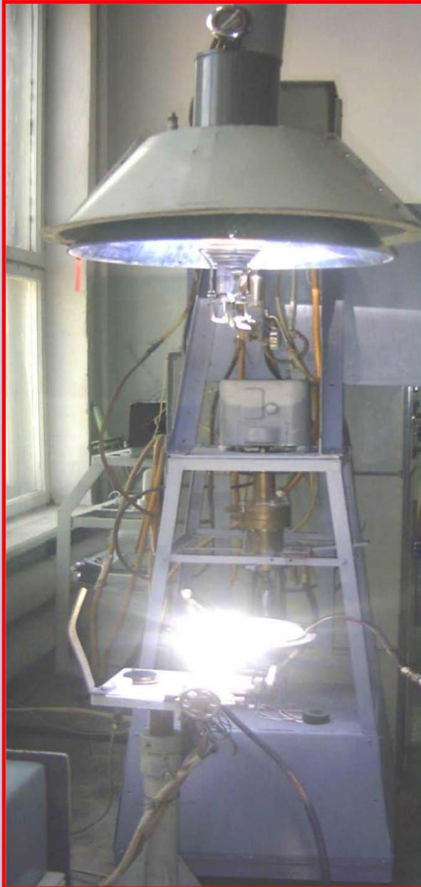
This installation allows to generate a focused beam with the radiation energy of density up to  $6 \cdot 10^6 \text{ W/m}^2$  on 12 mm diameter spot
