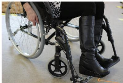
The Neater Uni-wheelchair steering mechanism
