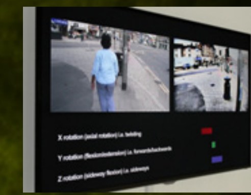
X, Y and Z rotation data is synchronised with the video, to determine the amplification of the video effects.
