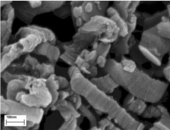
$NH_2$ -functionalized CNF-PL after shear mixing
