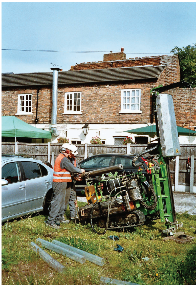
Figure 15.4: Windowless-sampling rig in operation: getting permission from many land-owners was a major problem. Note the steel liner and Perspex sleeves
