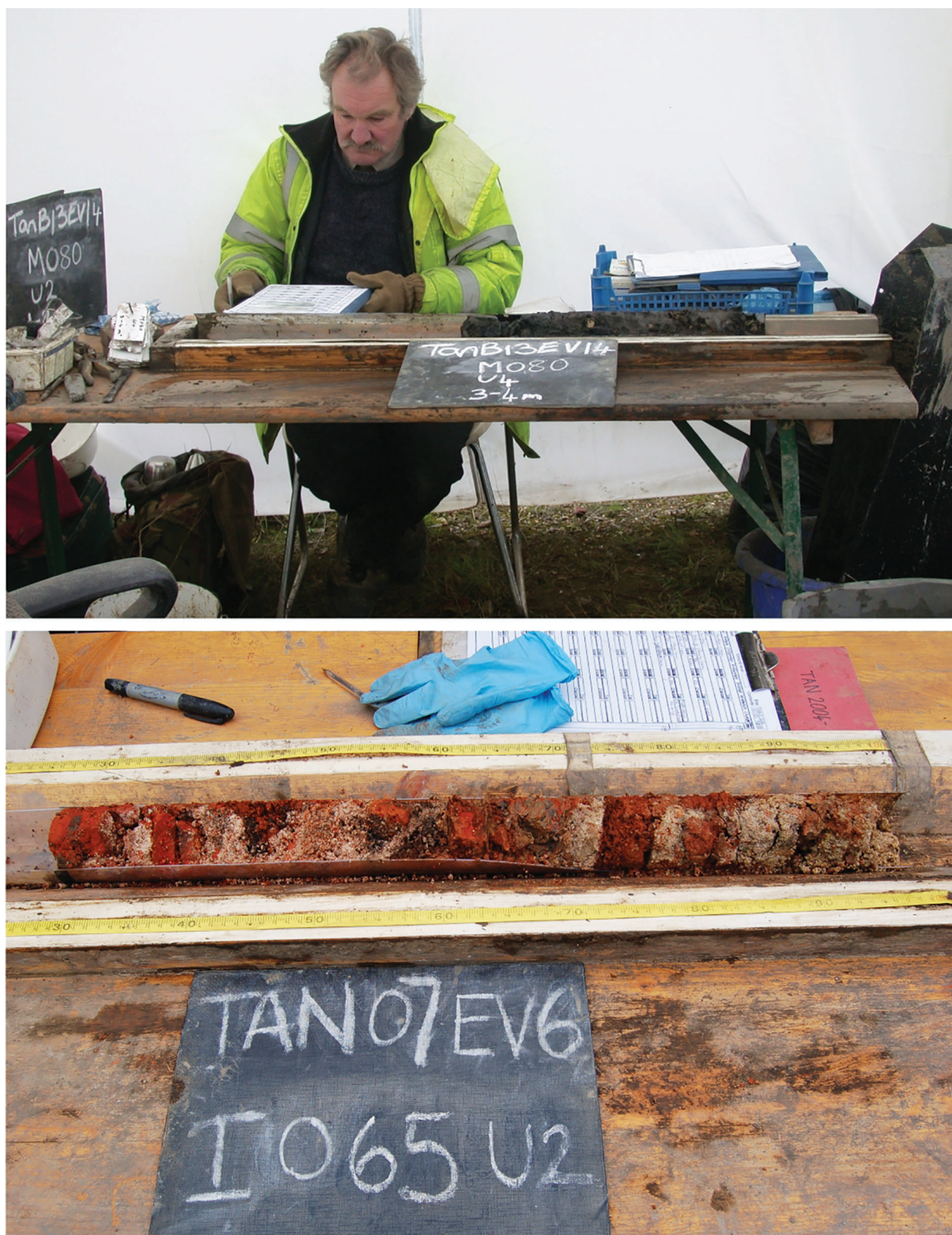
Figure 14.4: Logging table and a detail of its trough, holding a windowless-sample of a Roman wall
