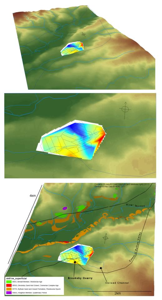
*Figure 3.5a-c: Further work undertaken at Brooksby quarry by drilling boreholes and electrical tomography to further refine channel through the rockhead*
