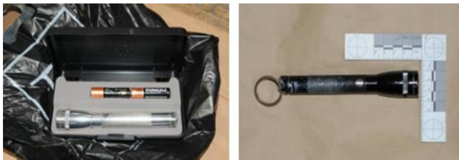
Figure 5. Mini torches converted into a firearm
